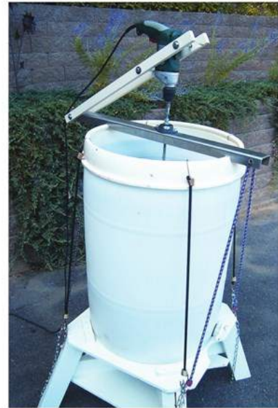
Beekeepers in their second and third years often build their own equipment. This is a home-made extractor from Ed Simon's book Bee Equipment Essentials.
