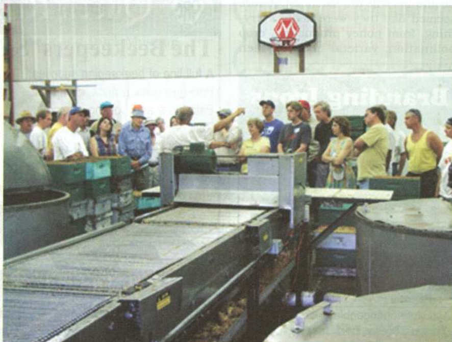
Jim Baerwald of Michigan demonstrates a multiple extractor uncapping facility for his commercial operation.
