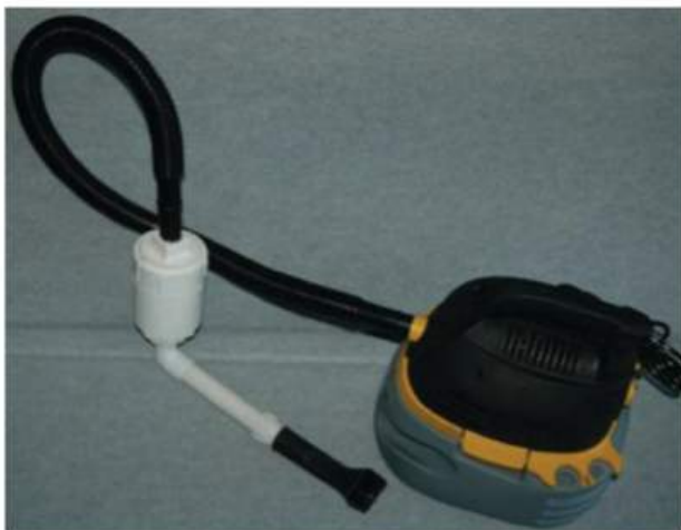
Fig. 1. The Dust-ructor is a shop vac with a hose modified to pass through a PVC chamber accommodating 120 g powdered sugar.
