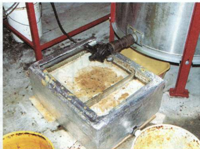
Insulated sump holds honey so it may be pumped into the buckets a few at a time.
